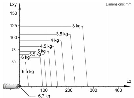
The KR 6 R900-2 is designed for a rated payload of 6 kg in order to optimize the dynamic performance of the robot. With reduced load center distances and favorable supplementary loads, a maximum payload of up to 6.7 kg can be mounted. The specific KUKA Load case must be verified using KUKA. For further consultation, please contact KUKA Service.
