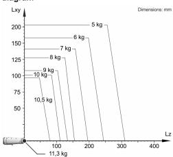
The KR 10 R900-2 is designed for a rated payload of 10 kg in order to optimize the dynamic performance of the robot. With reduced load center distances and favorable supplementary loads, a maximum payload of up to 11.3 kg can be mounted. The specific KUKA Load case must be verified using KUKA. For further consultation, please contact KUKA Service.
