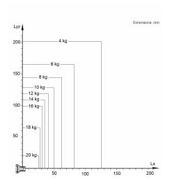
The KR 20 R1000 Z450 is designed for a rated payload of 10 kg in order to optimize the dynamic performance of the manipulator. With the reduced load center distances, higher loads up to the maximum payload may be used. The specific load case must be verified using KUKA.Load. For further consultation, please contact KUKA Support.
