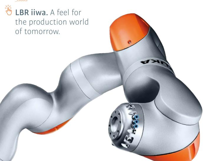
With the arrival of the LBR iiwa – one of KUKA's lightweight cobots specializing in sensitive assembly work – safety fences make way for human-robot collaboration in the workspace.
