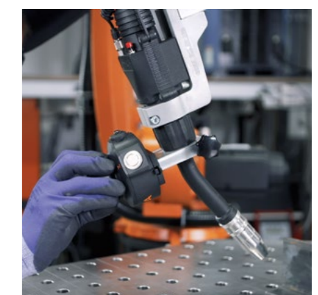
The path points are addressed by means of manual guidance directly at the torch during welding. Context-specific welding and motion commands can be entered using the buttons on the 6D mouse.
