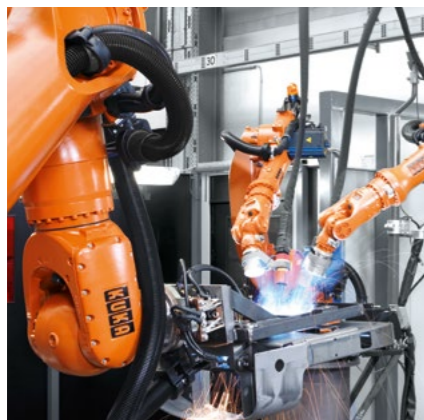
Jigless welding in commercial vehicle production: the handling robot positions the workpiece for welding by the two welding robots.
